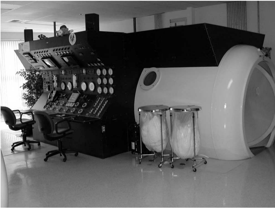
Fig. 3. Multiplace hyperbaric oxygen chamber (outside). (Courtesy of Kindred Hospital, Las Vegas, NV.)
