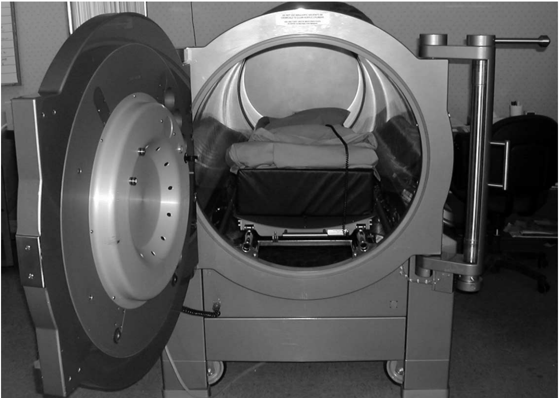
Fig. 1. Monoplace hyperbaric oxygen chamber. (Courtesy of Sunrise Hospital and Medical Center, Las Vegas, NV.)
